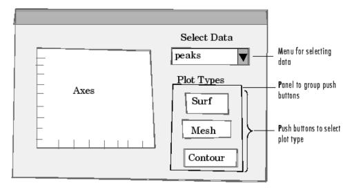
A panel contains three push buttons that enable you to choose the type of plot you want. The pop-up menu contains three strings—peaks, membrane, and sinc, which correspond to MATLAB functions and generate data to plot. You can select the data to plot from this menu.
