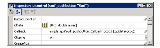
simple\_gui is the name of the GUI M-file as well as the name of the main function for that GUI. The remaining arguments generate input arguments for pushbutton1\_Callback. Specifically,
