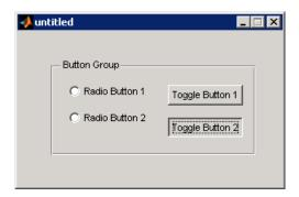
The button group's SelectionChangeFcn callback is called whenever a selection is made. Its hObject input argument contains the handle of the selected radio button or toggle button.
