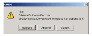
**6** If you chose to activate the GUI by selecting **Run** from the **Tools** menu or by clicking the **Run** button ▶ on the toolbar, and if the directory in which you save the GUI is not on the MATLAB path, GUIDE opens a dialog box, giving you the option of changing the current working directory to the directory containing the GUI files, or adding that directory to the top or bottom of the MATLAB path.
