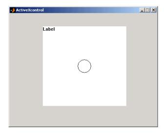
3 View the ActiveX Properties with the Property Inspector. Select the control in the Layout Editor, and then select Property Inspector from the View menu or by clicking the **Property Inspector** button on the toolbar.
