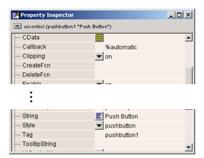
When you save the GUI, GUIDE constructs the name of the callback by appending an underscore (\_) and the name of the callback property to the value of the component's Tag property. For example, the MATLAB expression for the Callback property for a push button in the GUI simple\_gui with Tag property pushbutton1 is
