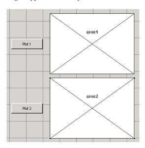
1 Add this code to the **Plot** 1 push button's Callback callback. The surf function produces a 3-D shaded surface plot. The peaks function returns a square matrix obtained by translating and scaling Gaussian distributions.
