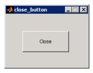
This is the push button's Callback callback. It displays the string Goodbye at the command line and then closes the GUI.
