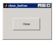
This is the push button's Callback callback. It displays the string Goodbye at the command line and then closes the GUI.
