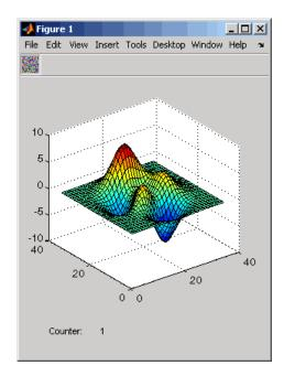
**3** Continue clicking the toggle tool to toggle between surf and mesh plots of the peaks data.
