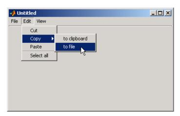
When a user selects **Edit > Copy > to file**, no **Copy** callback is needed to perform the action. Only the Callback callback associated with the **to file** item is required.
