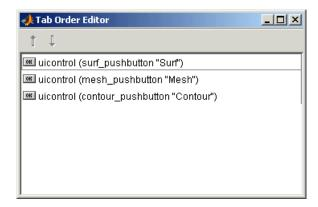
The Tab Order Editor displays the panel's components in their current tab order. To change the tab order, select a component and press the up or down arrow to move the component up or down in the list. If you set the tab order for the three components in the example to be
