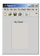
The Parent property specifies the handle fh of the parent figure. You can also specify the parent as a panel or button group.
