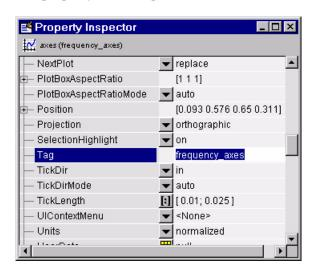
For example, the Tag of the axes used to display the FFT is set to frequency axes. Therefore, within a callback, you access its handle with
