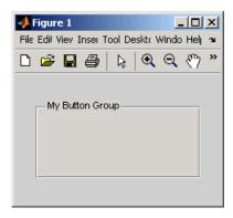
The Parent property specifies the handle fh of the parent figure. You can also specify the parent as a panel or button group.
