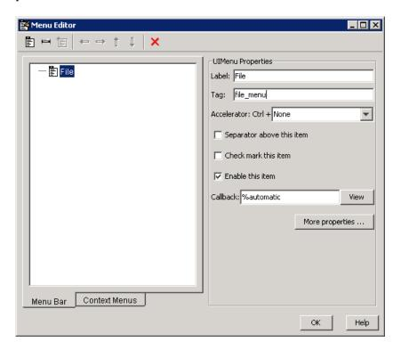
3 Fill in the **Label** and **Tag** fields for the menu. For example, set **Label** to File and set **Tag** to file\_menu. Click outside the field for the change to take effect.
