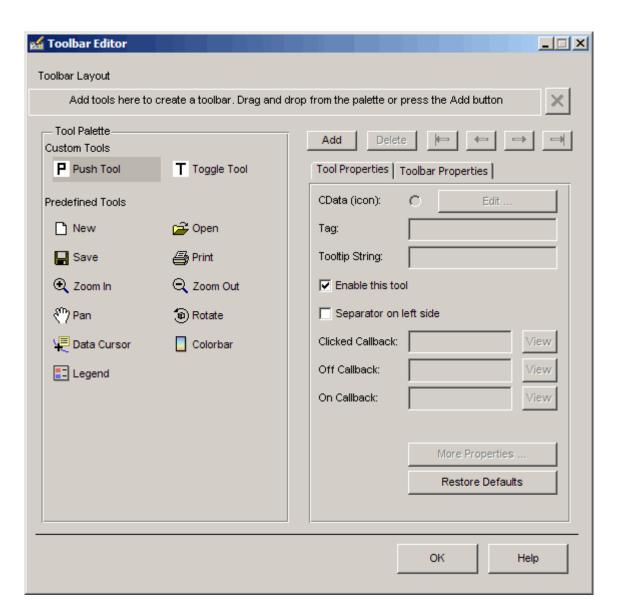
To add a tool, drag an icon from the **Tool Palette** into the **Toolbar Layout** (which initially contains the text prompt shown above), and edit the tool's properties in the **Tool Properties** pane.
